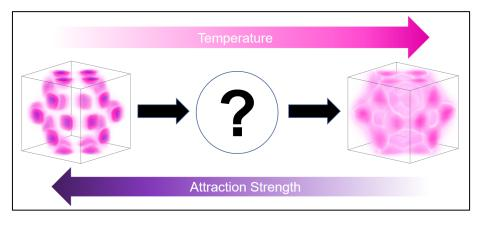
Average visitation frequency of the small particle sublattice in a BCC unit cell. The sublattice is localized at low temperatures and large number of grafted chains per small particle (proxy for interaction strength) and delocalized at high temperatures and lower number of grafted chains.
