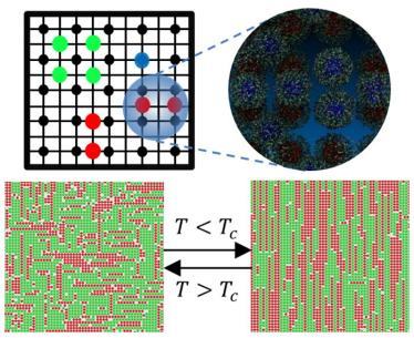
Top: Schematic diagrams of the MC model (left) and the MD model (right); Bottom: Orientational disordered– ordered phase transition as a function of temperature.
