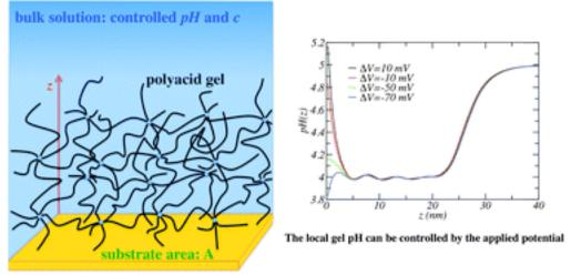
In this work, we used a Molecular Theory to study the response of a thin film of crosslinked hydrophilic polyacid chains to variations in external stimuli such as pH, salt concentration and applied electric potential.
