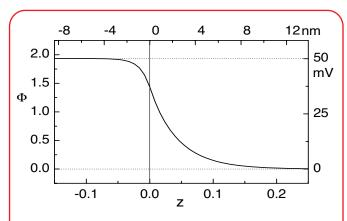
Plot of the electrostatic potential for the system of a membrane separating the two chemically distinct regions with different salt concentrations, similar to those found in physiological systems. The distribution potential  $\Phi_{\rm D}$  is 1.93 in dimensionless units (50 mV); dimensionless and mV scales are shown at left and right sides of the above plot, respectively. The horizontal scale is shown in dimensionless units at bottom, and in nanometers on top.
