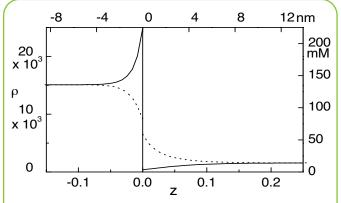
Plots the number density of ions in a system separating two regions with different salt concentrations, similar to those found in physiological systems. The concentration of positive ions is shown in a solid line, and for negative ions in a dotted line. Dimensionless and mM scales are shown at left and right. The horizontal scale is shown in dimensionless units at bottom of the plot and in units of nanometers on the top.
