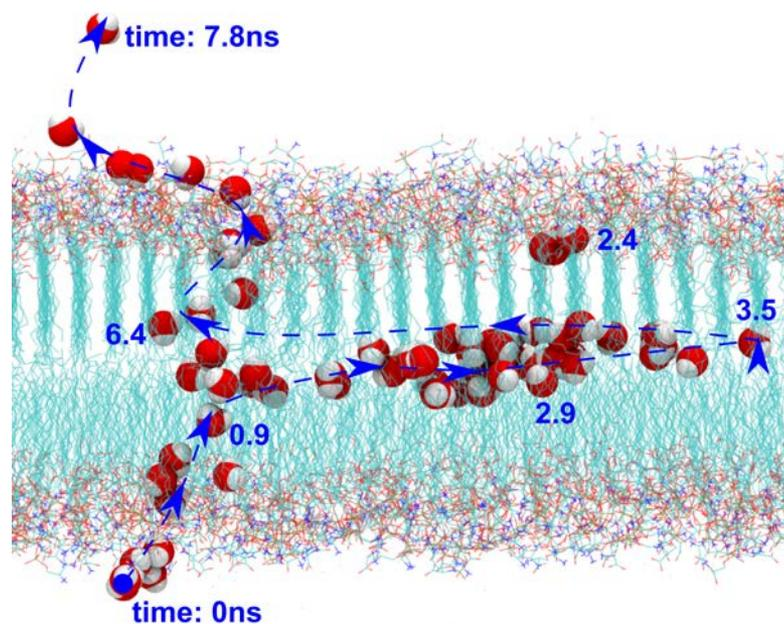
**Figure:** The permeation process of a single water molecule (highlighted) across a DLPS membrane. The trajectory of this water molecule within 7.8 ns is drawn in the same illustration with the dashed line to guide the eyes and some typical occupations labeled with the time. The other water molecules are removed for clarity..
